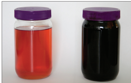
No. 2 heating oil (left) generates 93% less soot than No. 6 heating oil (right).
